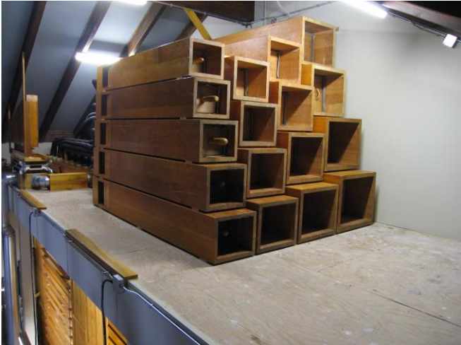
The 32' Contra Bourdon installed on shelf above organ
